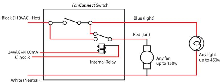
Inside the FanConnect™ switch is a 24VAC relay to control the 110VAC bath fan.
